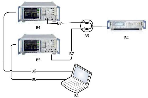
**Figure 3** Measurement Setup 2 (two), B1 – Portable Computer, B2 – Signal Generator (ASK generator), B3 – Signal Splitter, B4,B5 – Spectrum Analyzers, B6 – Ethernet Connection (Double Port Ethernet Card), B7 – SMA Cable
