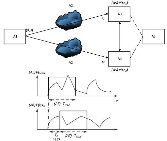
**Figure 7** Measurement Campaign Scenario for Cognitive Radio. A1 – Base Station, A2 – Obstacles, A3 - Sensor ( $SA_1$ ) with  $P(t,s_1)$ , A4 - Sensor ( $SA_2$ ) with  $P(t,s_2)$ , A5 – Computer. The distance between sensors is less than 200 meters.
