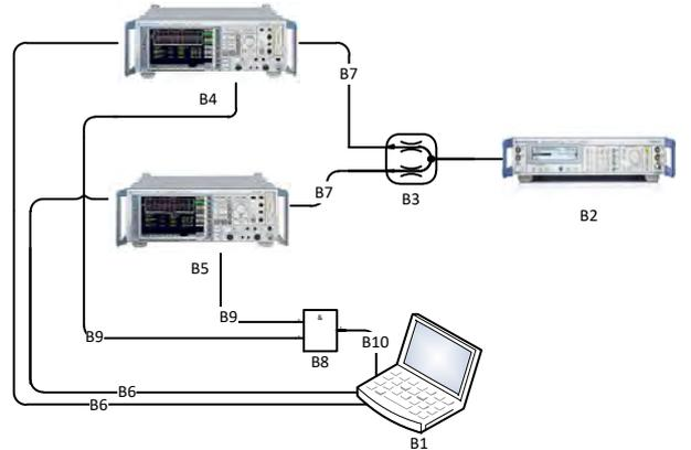
**Figure 4** Measurement Setup 3 (three), B1 – Portable Computer, B2 – Signal Generator (ASK generator), B3 – Signal Splitter, B4,B5 – Spectrum Analyzers, B6 – Ethernet Connection (Double Port Ethernet Card), B7 – SMA Cable, B8 – Card of TTL digital outputs commanded and Power supplied by USB (Universal Serial Bus), B9 – Cable connected to the trigger input of the Spectrum Analyzer, B10 – USB Cable
