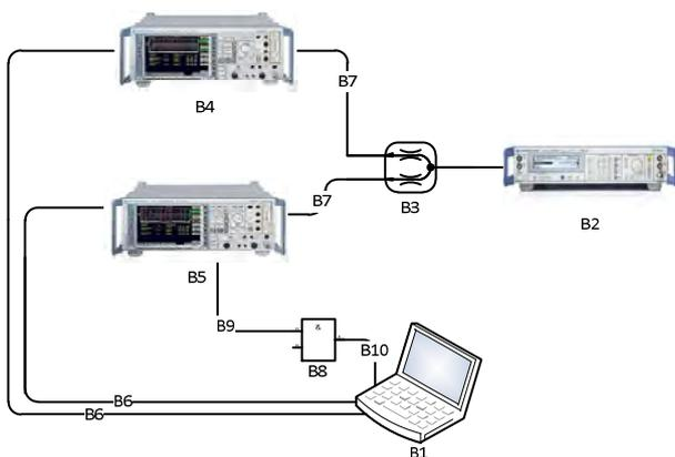
**Figure 2** Measurement Setup 1 (one), B1– Portable Computer, B2 – Signal Generator (ASK generator), B3 – Signal Splitter, B4, B5 – Spectrum Analyzers, B6 – Ethernet Connection (Double Port Ethernet Card), B7 – SMA Cable, B8 – Card of TTL digital outputs commanded and Power supplied by USB (Universal Serial Bus), B9 – Cable connected to the trigger input of the Spectrum Analyzer, B10 – USB Cable.
